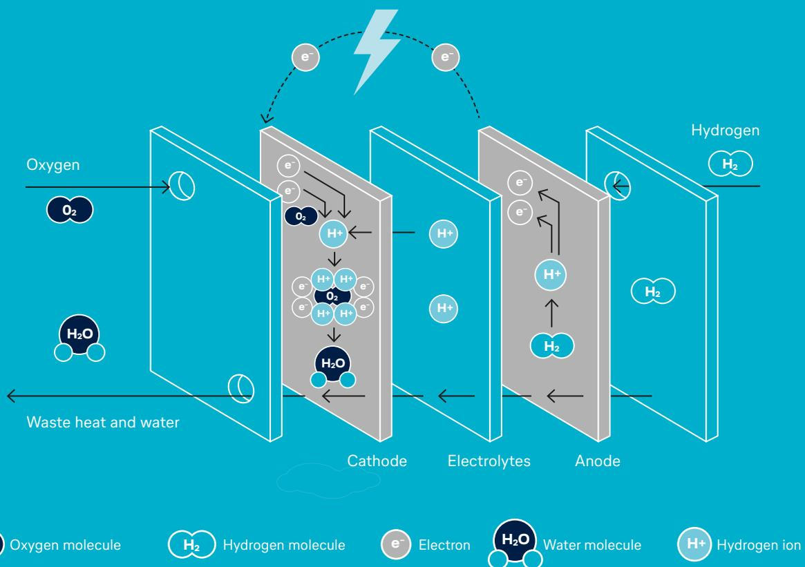
1. Each fuel cell contains two plate-shaped electrodes (anode and cathode) separated by an electrolyte. The electrolyte can conduct ions but is impermeable to gases. The catalyst materials on the electrodes ensure that the supplied gases release ions. Hydrogen molecules ( $H_2$ ) decompose at the anode into hydrogen atoms, which in turn become positively charged hydrogen ions ( $H^+$ ) by releasing electrons.
